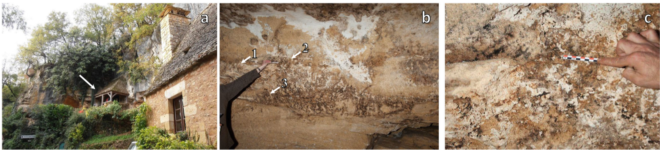
Fig. 1 The Sorcerer's cave (Saint-Cirq-du-Bugue, Dordogne, France): a entrance (white arrow); b sampling areas 1, 2 and 3; c enlarged view of the sampling area no. 2 showing gypsum efflorescences. Credit photo: LRMH
