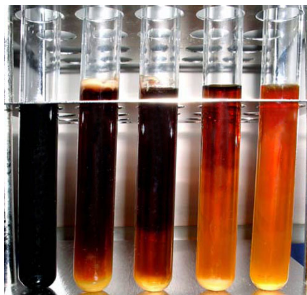
Fig. 4 Decolorization of azo dye, Remazol Black B by Halomonas sp. D2. From left to right: the first tube contains decolorization medium without inoculation; the others are inoculated decolorization media at time intervals of 24, 48, 72 and 96 h of incubation, respectively
