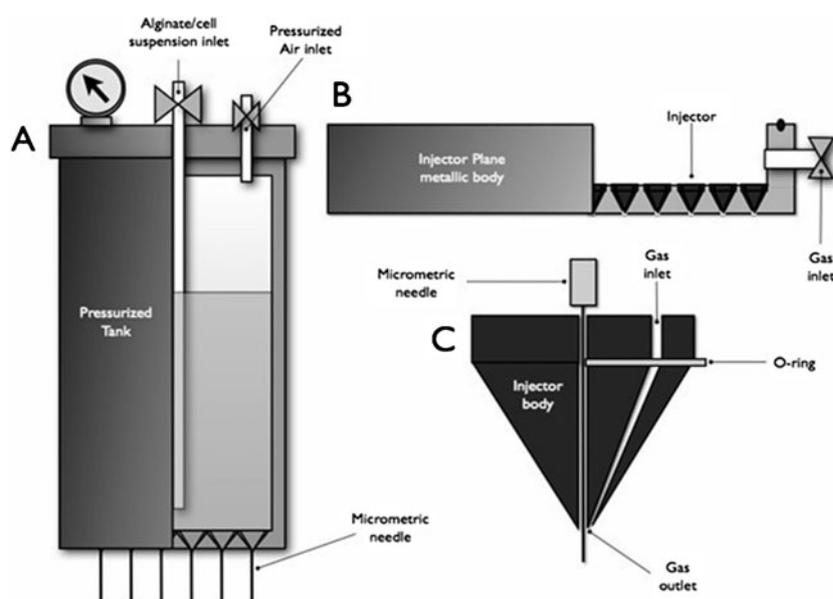
**Fig. 2** Diagram of the apparatus for the deposition of gaseous methyltriethoxysilane (MTES) on alginate beads
