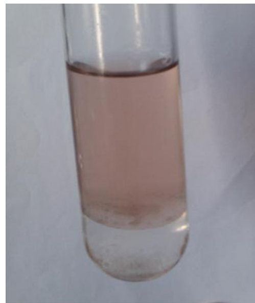
Fig. 5 Lilac pigment of TD16 extraction in aqueous two-phase system consisting of 20% PEG 1000/8% \text{KH}_2\text{PO}_3
