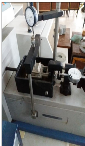
g. Vertical load application on sample
